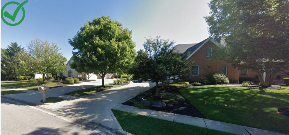
Where possible, place driveways side by side to create greater setbacks between homes
