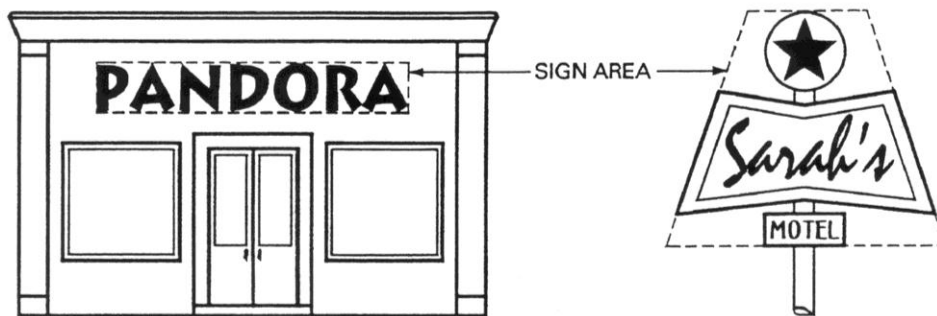
Figure 12-1: Illustration of calculating sign area.
