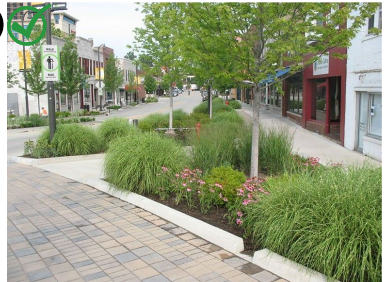
Heavily landscaped areas buffer pedestrian spaces from vehicular areas. Landscaping in front of commercial spaces should include a blend of shrubs, grasses and trees
