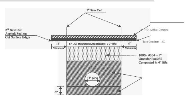
Note: The Pavement thickness indicated are indicated are minimum standards. If the pavement which is to be repaired has a greater thickness of asphalt, It shall be re placed in kind.
