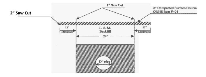
Gravel BacldiU ODTS Item 410 Typo A per County Water/Sewer Specification
